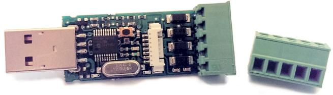
USB reader interface with Serial (TTL), Wiegand or Clock/Data interface
